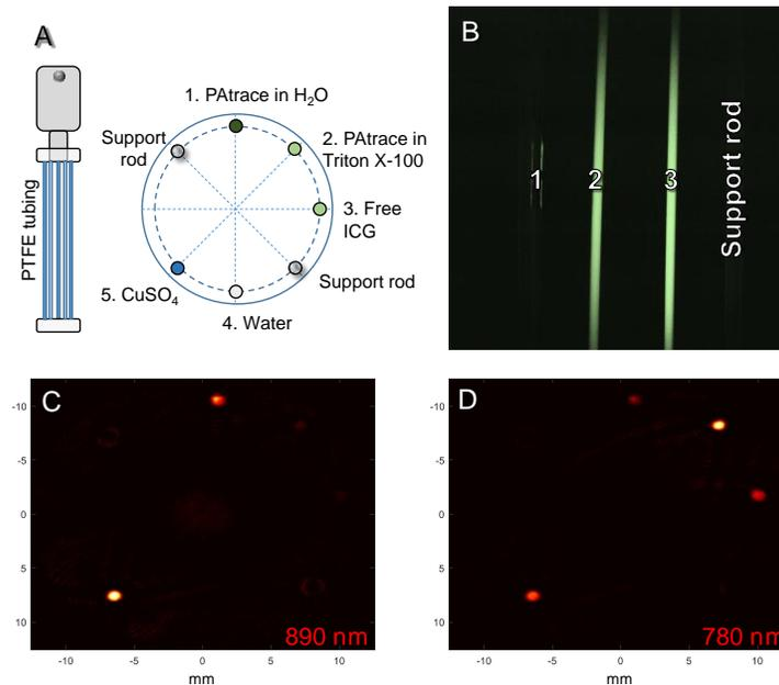
Figure 2. (A) Schematic of PAFT phantom design. On the left is the phantom, on the right is a horizontal slice view. (B) Fluorescence image showing tubes 1, 2, and 3, using 780 nm excitation. Tubes 4, 5, and support rods are not visible. (C) Horizontal slice view of PA at 890 nm. (D) Horizontal slice view of PA at 780 nm. The tubes' positions are matched in (A), (C), and (D) horizontal slices.
