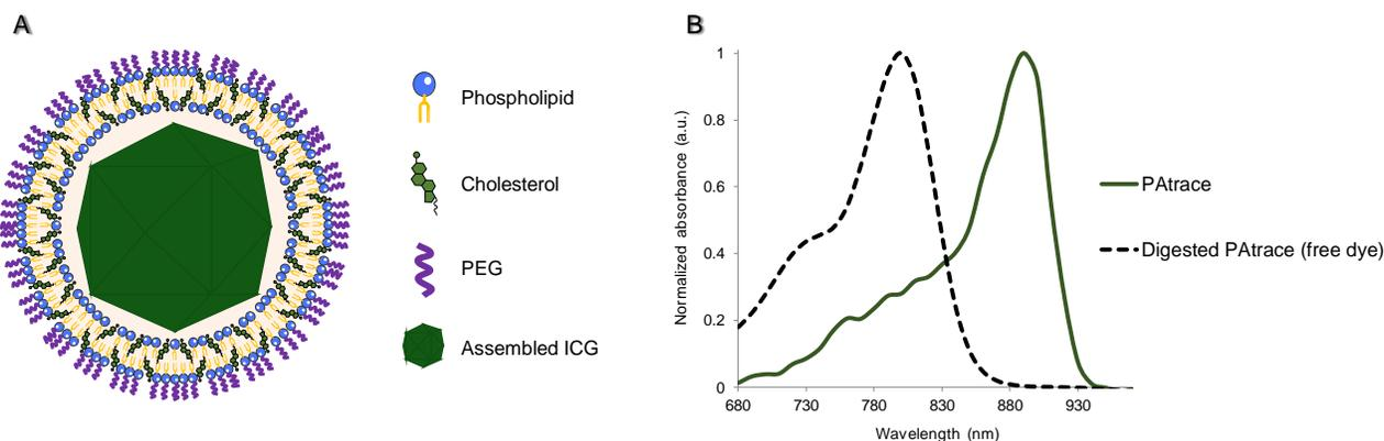
Figure 1. (A) Schematic of *PAtrace* shows an ICG J-aggregate encapsulated by a phospholipid and cholesterol shell. (B) Absorption spectra of intact and digested *PAtrace*. Before interaction, a sharp peak at 890 nm is obtained. After interaction with cells or environment, free ICG absorption spectrum is recovered.
