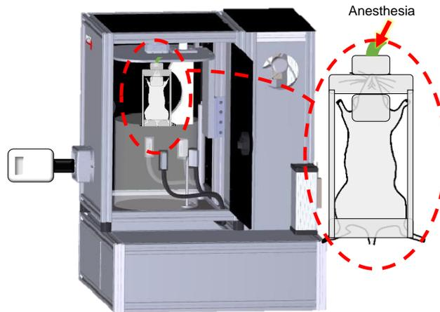
Figure 3. Schematic of mouse restrainer and its position in PAFT system.
